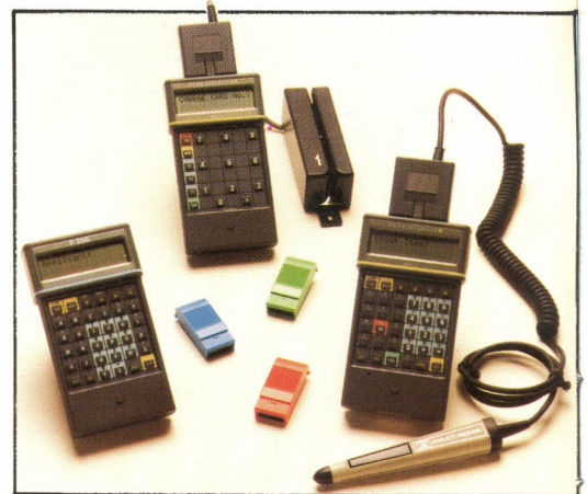
(l to r) The P250, POS 200 with magnetic card swipe reader, and Alpha POS with bar code reader.
