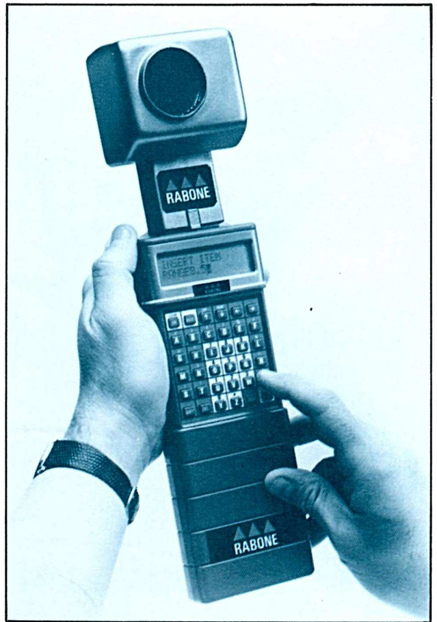
Rabone's new ultrasonic measuring systems for taking instant sonic measurements have a range of 0-15m and 0-30m with an accuracy of \pm 3mm .
