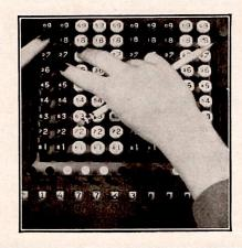
Hold 133 (the divisor) using small figures less one (132) directly over 147. Depress these divisor keys until the amount in the register dials at the base of the columns in which you are holding the divisor is less than 133.
