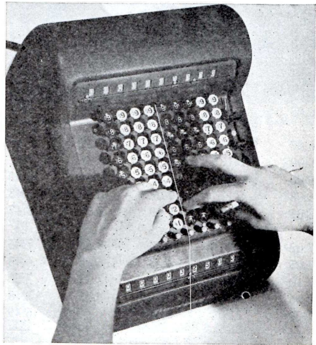
Unit position for multiplication over a fixed decimal point. Always hold the price on the keyboard, with dollars to the left of the fixed decimal point and cents to the right.
