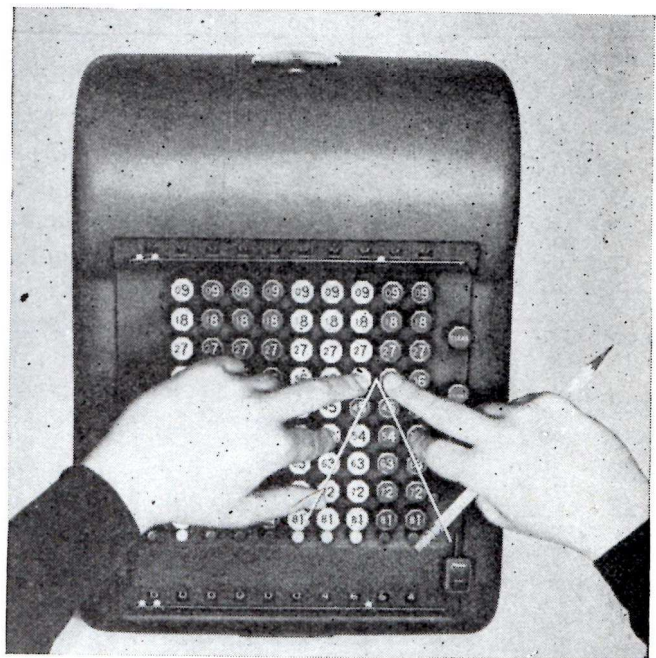
Position of fingers for holding reverse combinations such as 4664. The hands are turned in; both 4's are held with the first fingers; both 6's, with the second fingers. →
